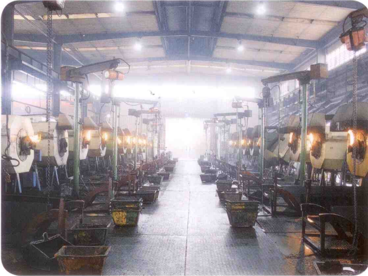
Rotary furnaces used in the heat treatment process provide a uniform heat for a more consistent and uniform result
