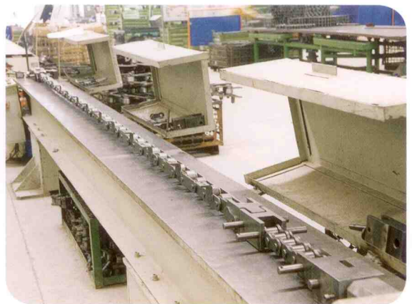
Pre-stressing after final assembly
