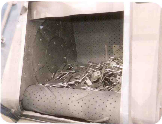
Shot peening improves fatigue strength and crack resistance
