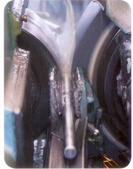
Pins are precision ground to enhance wear resistance and increase chain service life
